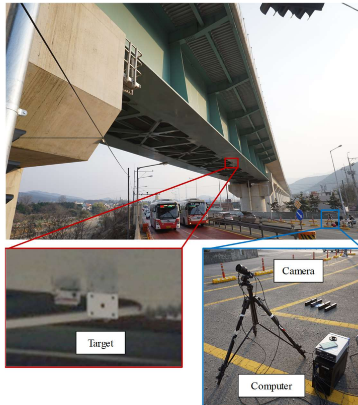
Figure 14. Field application of a computer vision-based method.
