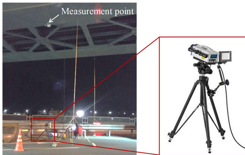
(a) Field application of LDV, a phase shift-based displacement sensor
