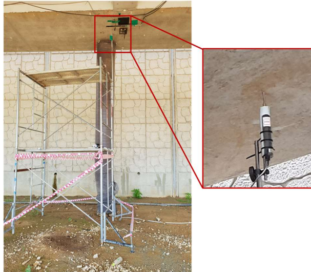
(a) Field application of LVDT
